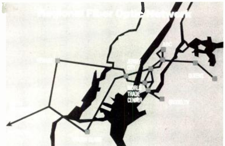
Map of New York City and New Jersey shows the extent of Teleport Communications's regional fiber optic network. Fully redundant, it provides access to common carriers and to Teleport's Staten Island satellite facility.
