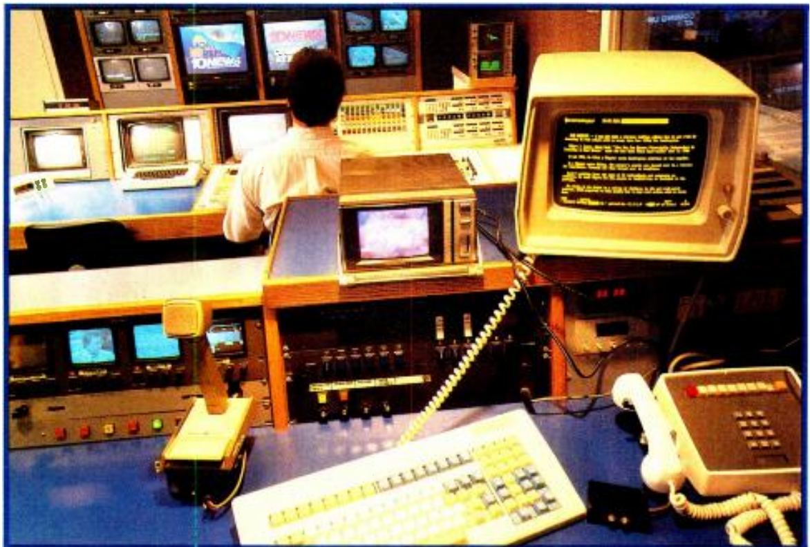
KGTV, in San Diego, produces news with the help of a Dynatech Newstar computer, Grass Valley Group 300 switcher, and an NEC DVE System 10.
